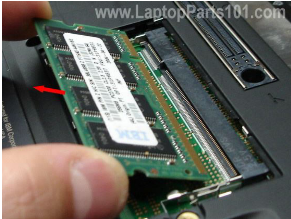
SODIMM and its slot
