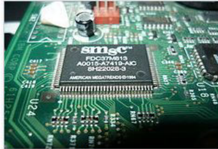
SMSC (now Microchip) Super I/O chip (FDC37M813) on IBM motherboard
