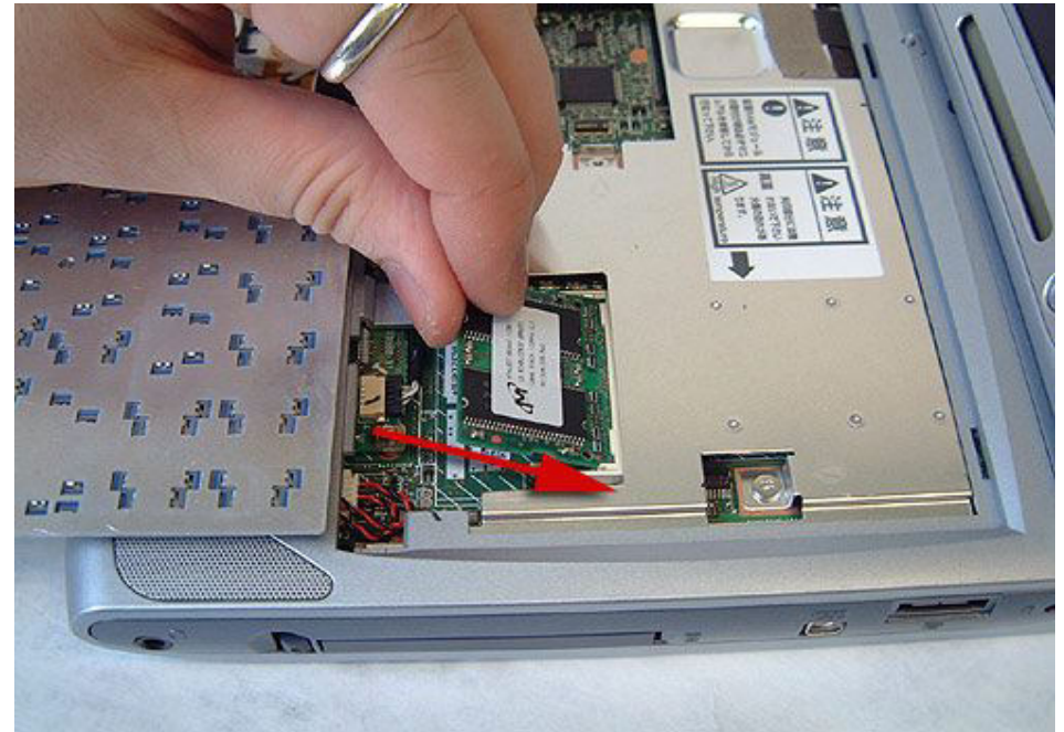
Micro DIMM and its slot
