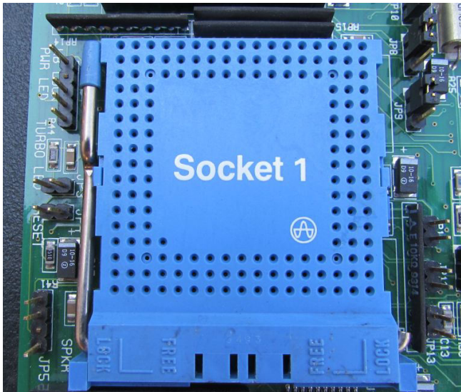
Socket 1 - for Intel 80486 PGA processors, with pin count 169
