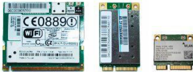
The traditional Mini PCI slot (shown first), the full height Mini PCIe slot (shown second) and the half height Mini PCIe slot (shown last)
