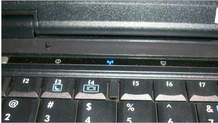
FIGURE 9.12 Network card toggle switch above the keyboard
