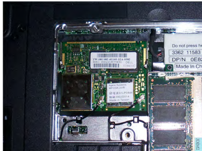
FIGURE 9.23 Mini PCI card installed in a laptop
