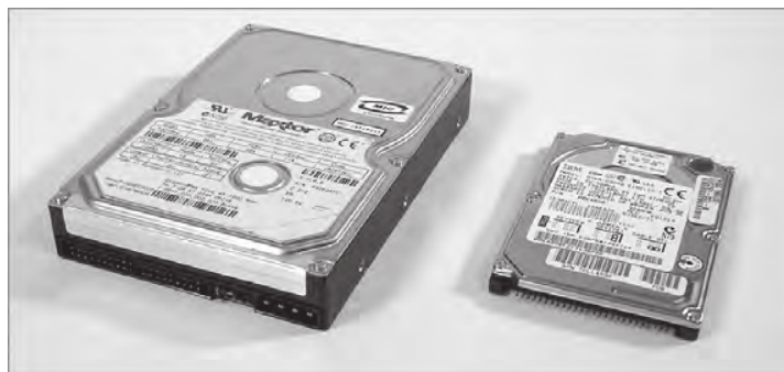
FIGURE 9.6 A desktop hard drive compared to a laptop hard drive
