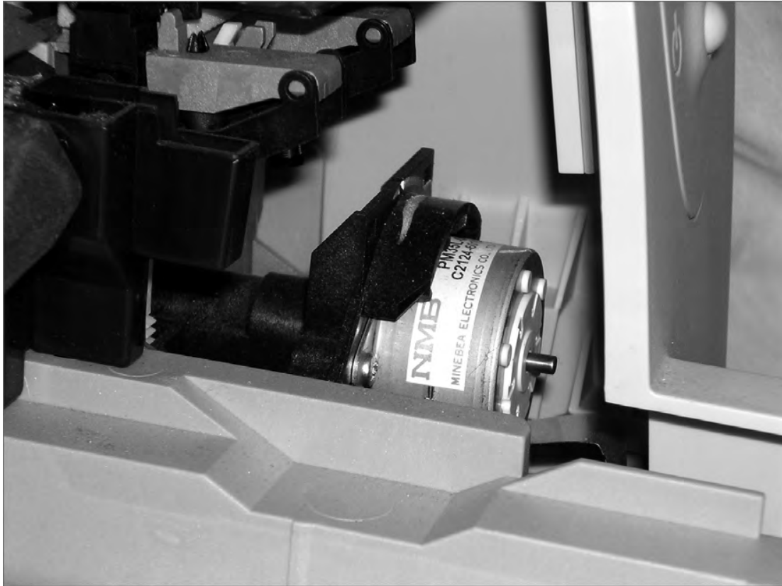
FIGURE 10.4 A carriage stepper motor
