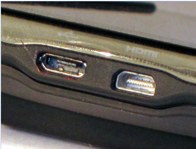
FIGURE 3.38 Type D HDMI interface
