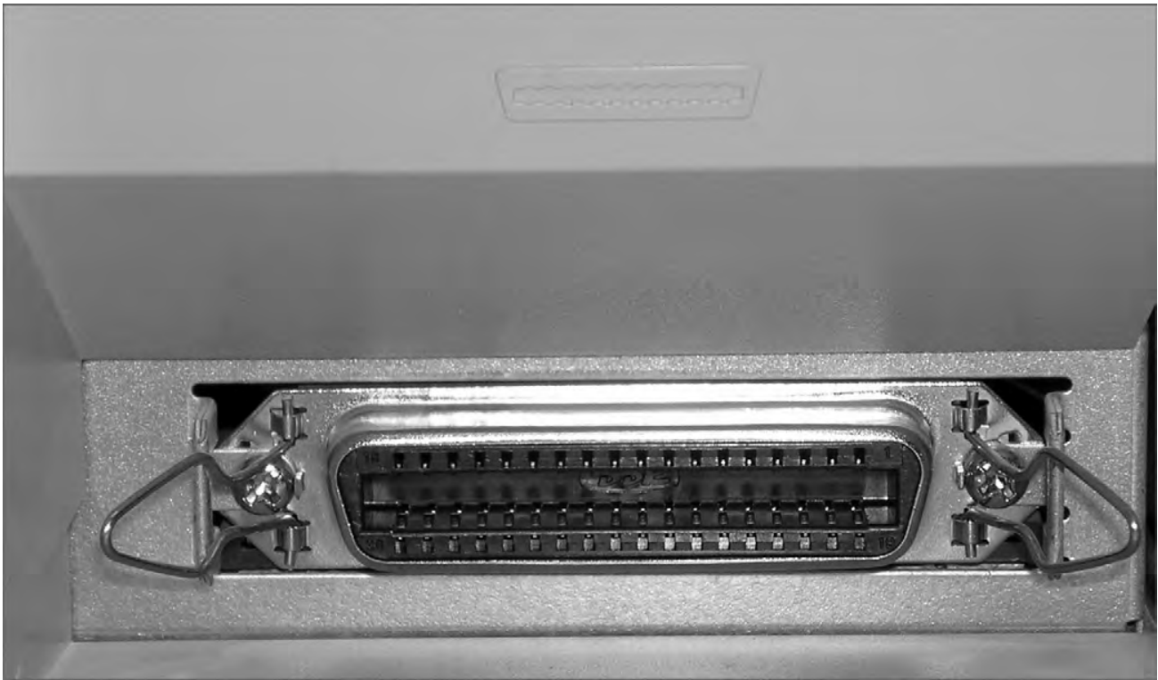
FIGURE 3.15 A Centronics connector
