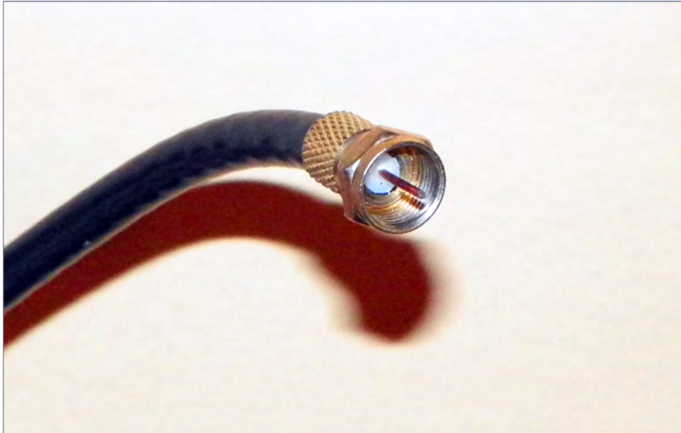
FIGURE 3.43 A CATV F connector and coaxial cable
