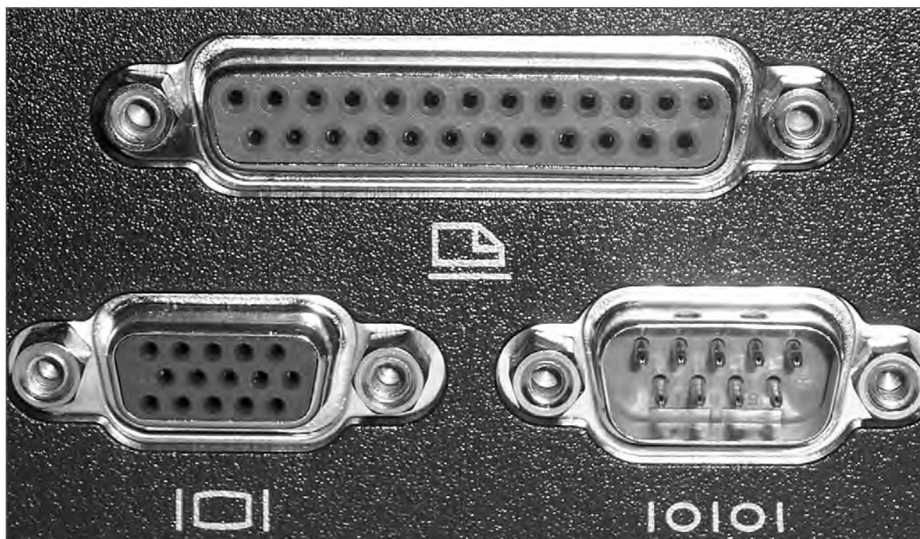
FIGURE 3.6 D-sub ports and connectors
