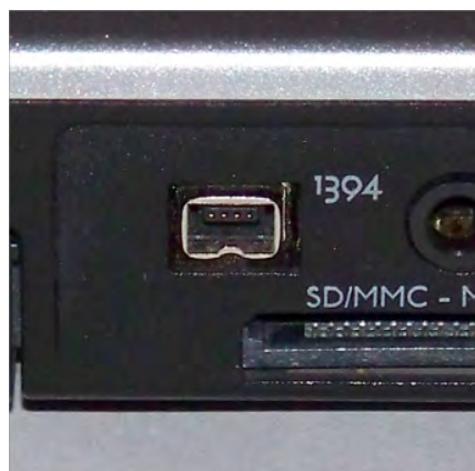
FIGURE 3.10 A 4-pin FireWire port on a laptop
