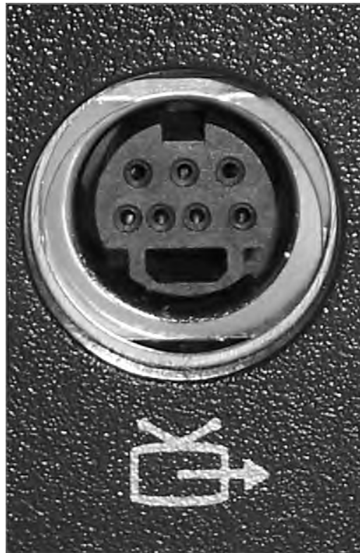
FIGURE 3.40 A 7-pin S-video port
