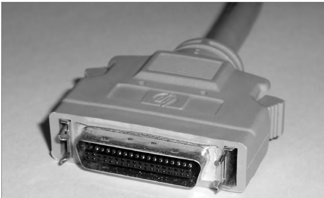
FIGURE 3.23 The mini-Centronics connector
