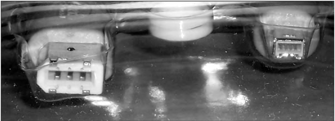
FIGURE 3.30 A FireWire (IEEE 1394) 6- to 4-pin alpha cable
