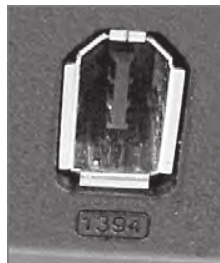
FIGURE 3.9 A 6-pin FireWire port on a PC
