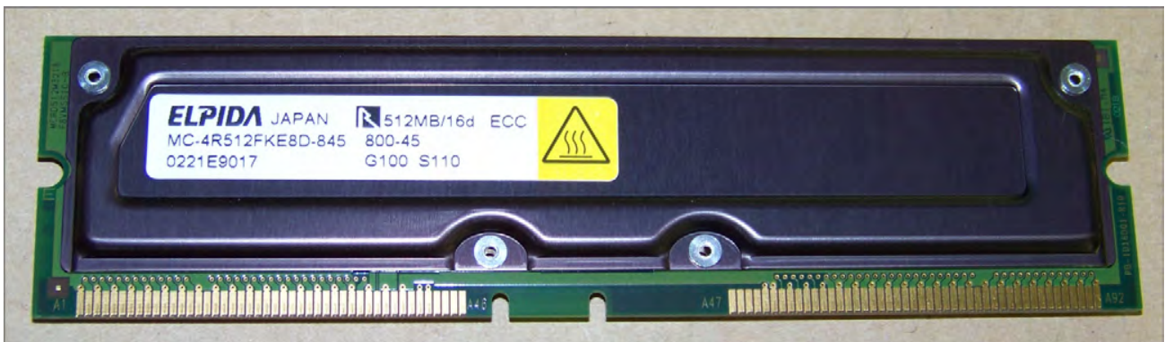
FIGURE 1.23 A Rambus RIMM module
