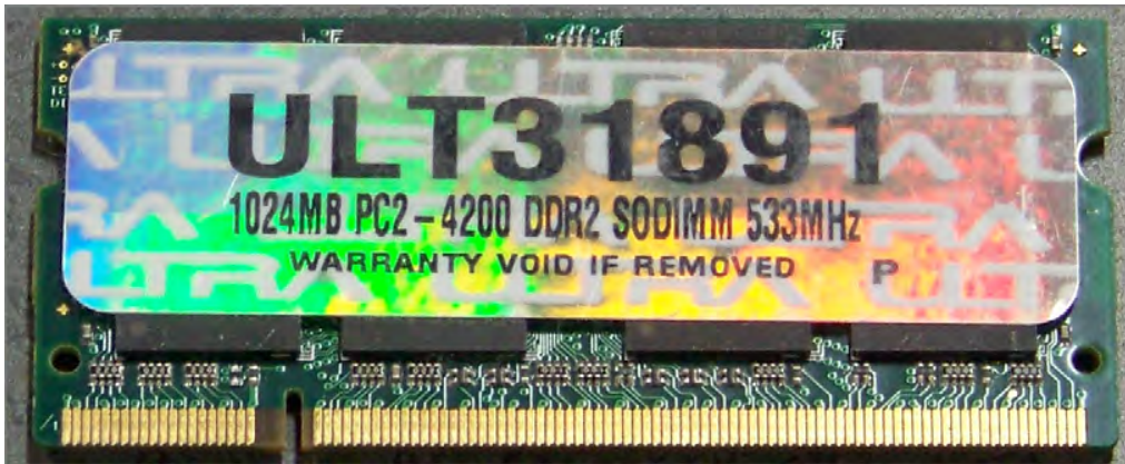
FIGURE 1.25 200-pin DDR2 SODIMM
