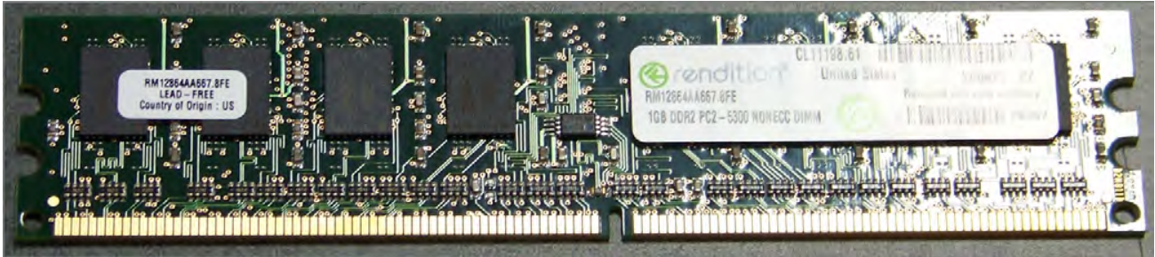
FIGURE 1.21 A DDR2 SDRAM module
