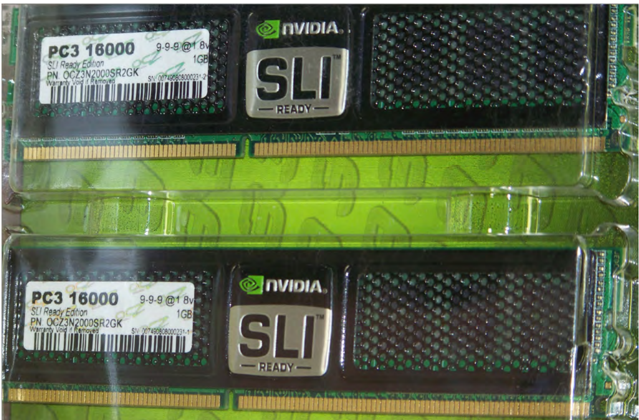
FIGURE 1.22 A pair of DDR3 SDRAM modules
